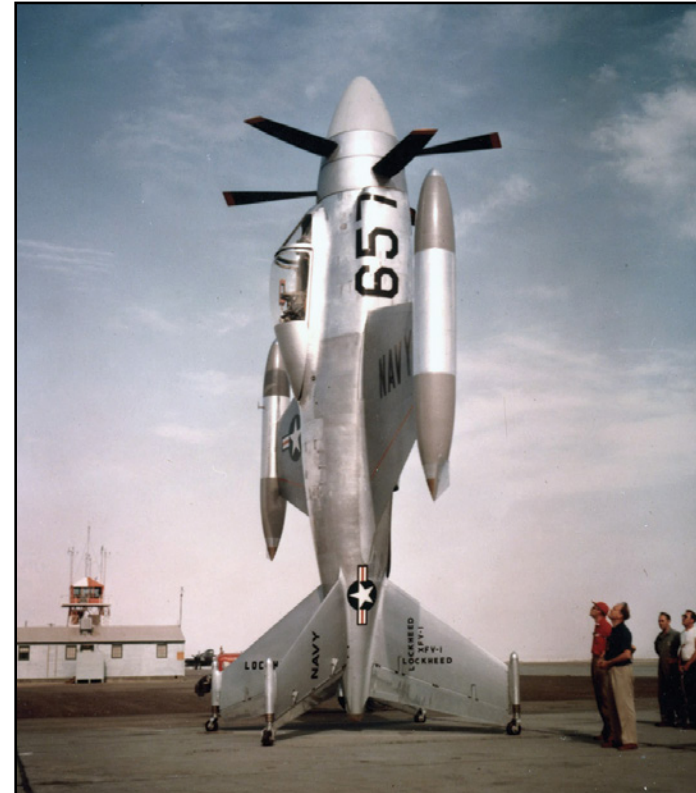
The XFV-1 pictured on its tail during evaluation of the VTOL aircraft in 1955. The aircraft featured contra-rotating propellers and was designed to take off and land vertically.
