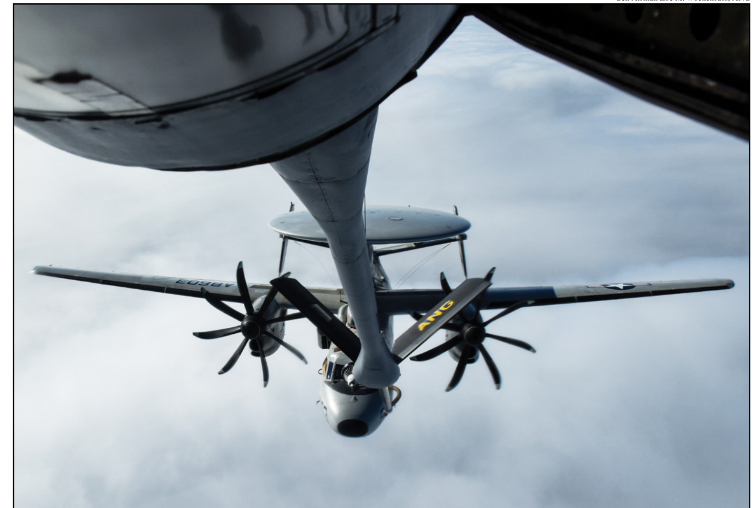
A VAW-126 Advanced Hawkeye refuels from a Pennsylvania Air National Guard KC-135 Stratotanker on 4 Feb '21. Tanking on this platform is the most challenging for E-2D aircrew.
